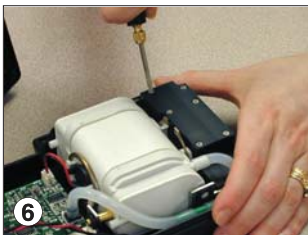
6 Remove 6 screws from housing plate.
