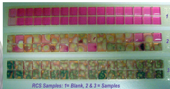
Figure 3. Viable air samples on agar strips taken with a Reuter Centrifugal Sampler (RCS).
