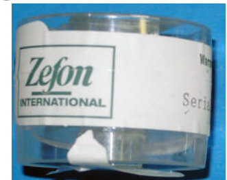
Figure 7. Air-O-Cell Cassette commonly used for non-viable air samples.
