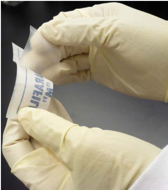
Peel the parafilm for sealing plates
